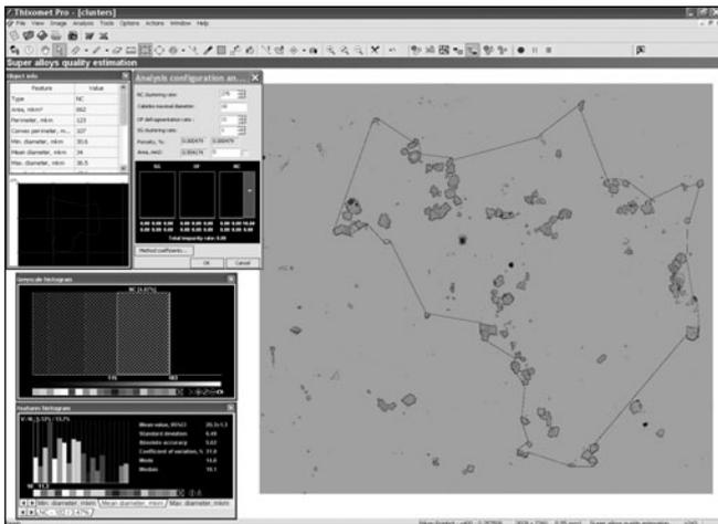
Fig.2. Thixomet screen. Estimation of impurity rate
