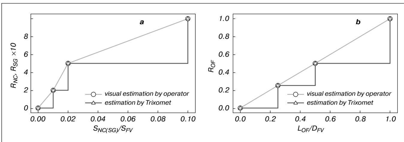
Fig. 1. Defect rate versus its dimension for nitride clusters, slag globule (a) and for oxide film (b)
