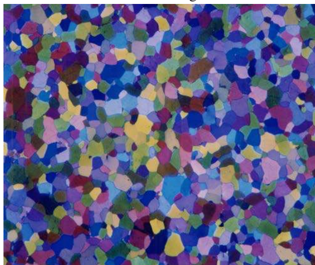
a) Motor Lamination Steel (original 100X)
