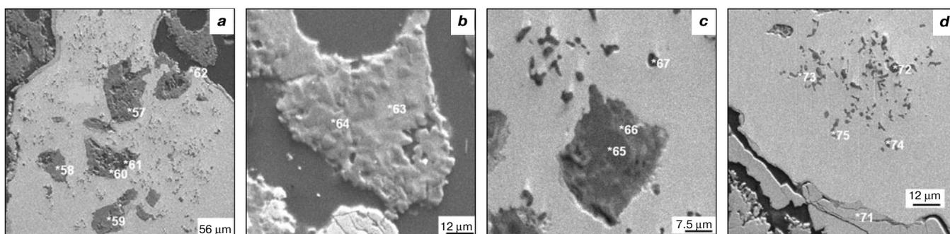
Fig. 2. Composition of nonmetallic inclusions in metallic beads
