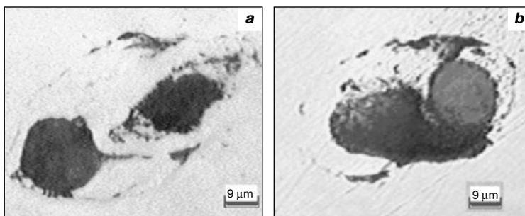
Fig. 3. The cavities around the nonmetallic inclusion after tensile test
