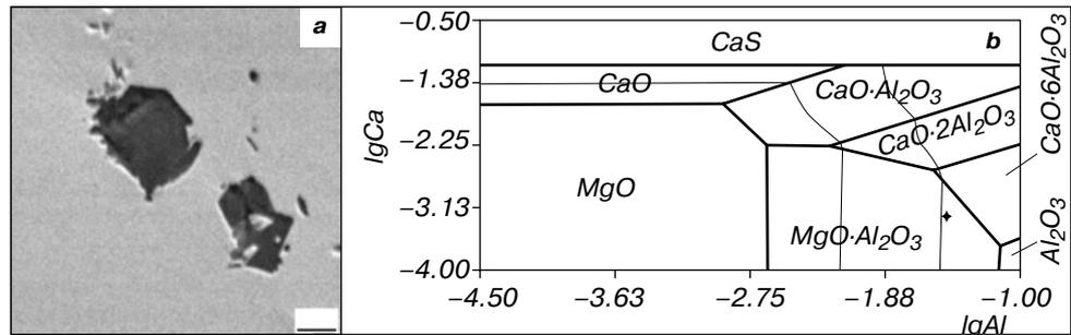
Fig. 7. Endogenous inclusions of magnesian spinel (a) and surface of component solubility in metal for Fe–0.07C–O–0.0005Mg–Ca–Al system at 1,550 °C (b)
