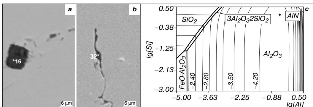
Fig. 8. Inclusions of  $\text{AlN}$  (a),  $3\text{Al}_2\text{O}_3\cdot 2\text{SiO}_2$  (b) in electric steel and surface of component solubility in metal for Fe–0.04C–0.25Mn–O–Si–Al system at 1,500 °C (c)
